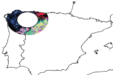
Figure 2.4: Compostilla II coal-fired power plant located in the center of the red circle (upper left) is a source of airborne Cu. CTPs of Cu were calculated using eq 2.7 for each of the 1-km grid cells representing soils from the HWSD database (FAO/IIASA/ISRIC/ISS-CAS/JRC 2012). The deposition area can be divided into subareas of circle (inner part) and torus shape (outer parts). The deposition of metal in each grid cell with subareas is calculated from the deposition function published in de Caritat et al. (1997). Insert in the upper right corner is Fig. 3 from de Caritat et al. (1997).
